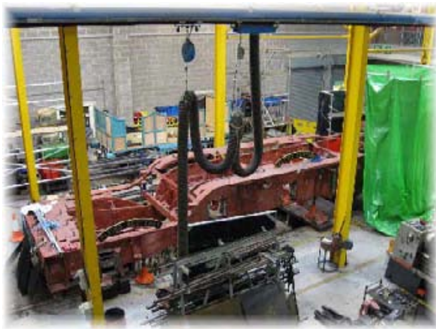
The Flying Scotsman's frame - straightened by over 1".
